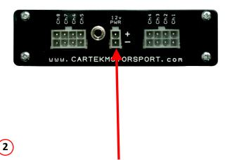
Whilst still holding both buttons connect power to the Relay Unit
